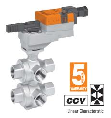
**Mode of Operation** The control valve is operated by an electronic actuator that responds to a modulating VDC/4...20 mA control signal. The actuator will then move the ball of the valve to the position dictated by the control signal thus changing the flow.
